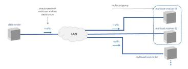
When it comes to power systems communication, IGMP protocol can be used when there is multicast communication between a Phasor Measurement Unit (PMU) and a Phasor Data Concentrator (PDC). With IGMP snooping, the receiver can send a "join group" to join an IP multicast group. To stop receiving data, the receiver sends a "leave group". Reason S20 has support to IGMPv1, IGMPv2 and IGMPv3 protocols.
