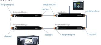
When using STP, only one path is available and transmits the network data. In the case of failure in any link between two Ethernet switches, the STP protocol recalculates the best path once again and after a short period of time the communication is reestablished. The time to recover the communication is also dependent on the STP protocol version.
